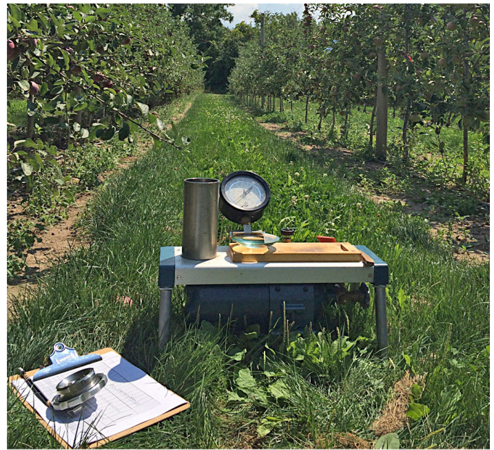
Figure 3. Pressure chamber used to assess tree water stress in the orchard.
